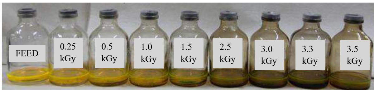
Fig. 4: PM567 feed and gamma radiolysed degraded dye at different absorbed doses (in ethanol)
