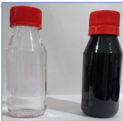
Photo 1: Formulated samples for the coating : Left sample is the transparent blend and right sample is the blend with the dye incorporated in it.
