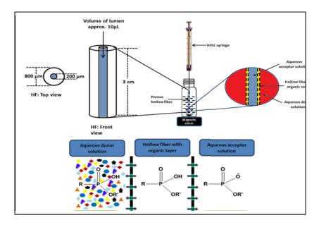
Passive diffusion the analytes across the pores of hollow fibre was a limiting factor of this method, it was overcome by development of a simple and fast method through microfluidic electromembrane extraction ( $\mu$ -EME). The edge provided by this method was efficiency (3 min) and sample size (10 micro liter).
